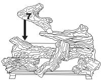
Figure 46 - Installing Log No. 7
